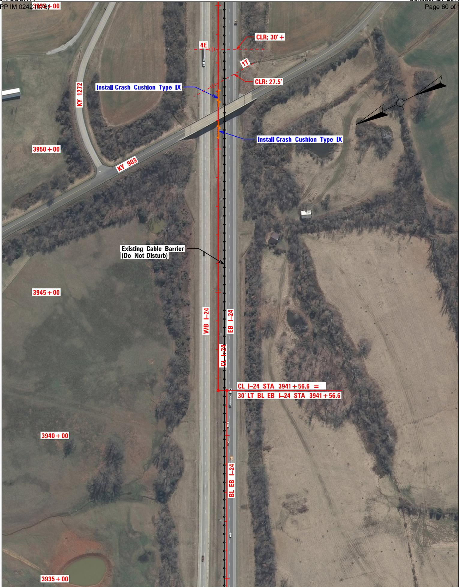
Eastbound I-24 Rehab Plan - Scale 1" = 200' - Sheet 18 of 19 - Sta 3935+00 To Sta 3955+00
