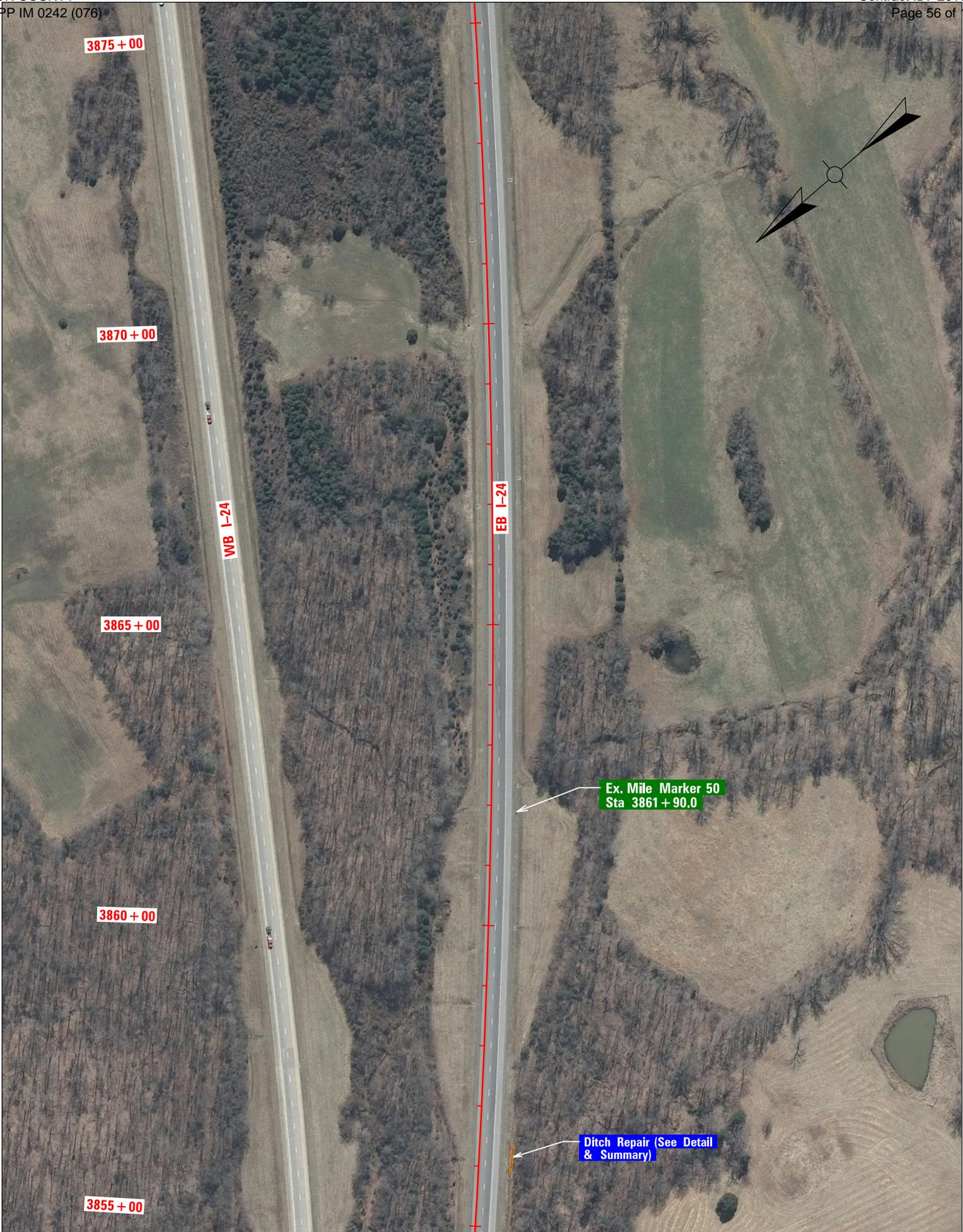
Eastbound I-24 Rehab Plan - Scale 1" = 200' - Sheet 14 of 19 - Sta 3855+00 To Sta 3875+00
